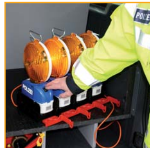
2. Switching on / synchronization
